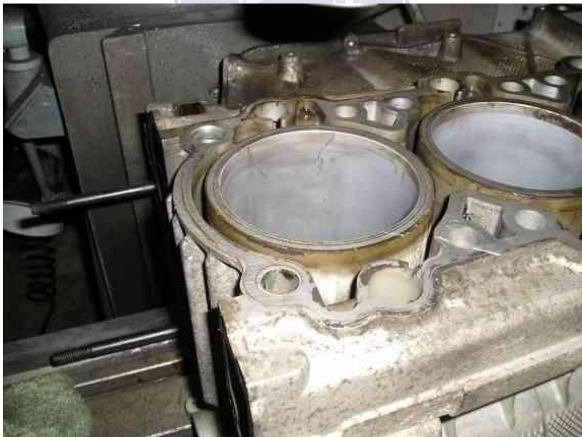
Cracks shown below leading to a chunk eventually breaking free.
