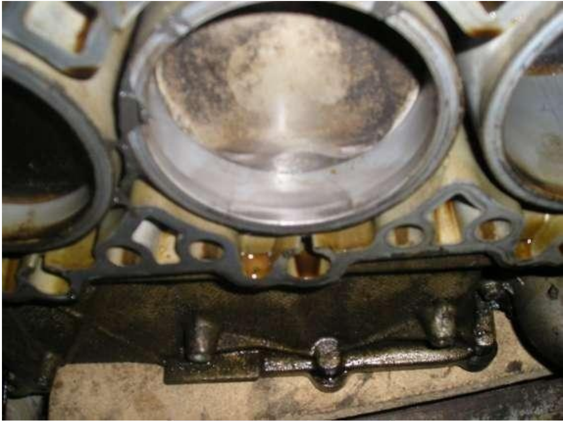
Picture showing a typical single cracked cylinder block
