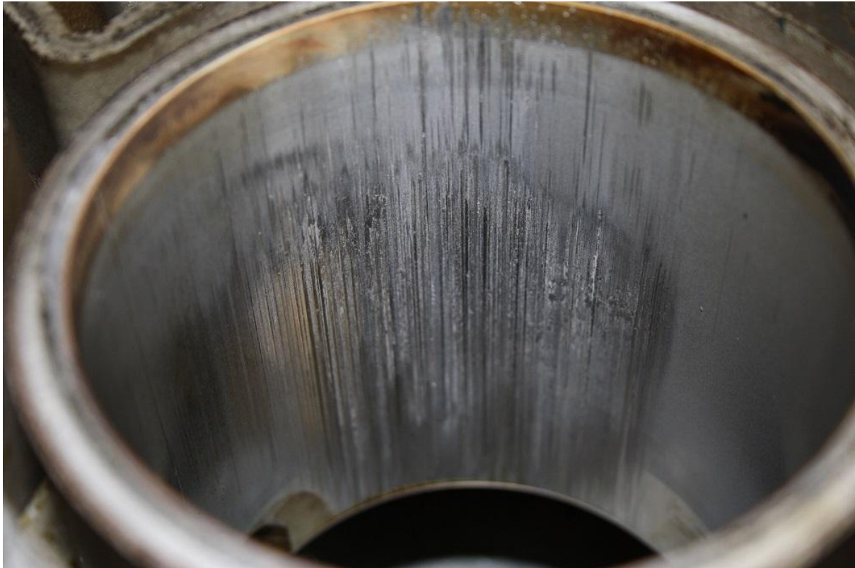
A typical scored piston (notice the black flecks in the surface).
